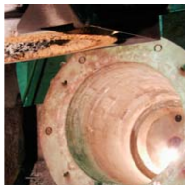
The furnace is to clean and the coil grout is to check
