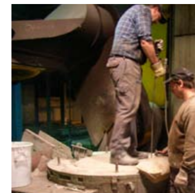
Fix the crucible with backup mix by using a backup mix vibrator.
